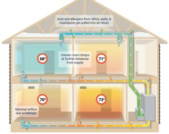
HVAC to your smart thermostat, none of them can do their job if your air vent system has invisible cracks, leaks and holes. In fact, the Department of Energy estimates that most homes leak 25-40%, resulting in higher energy bills, contaminated air and hot and cold zones in your home.
